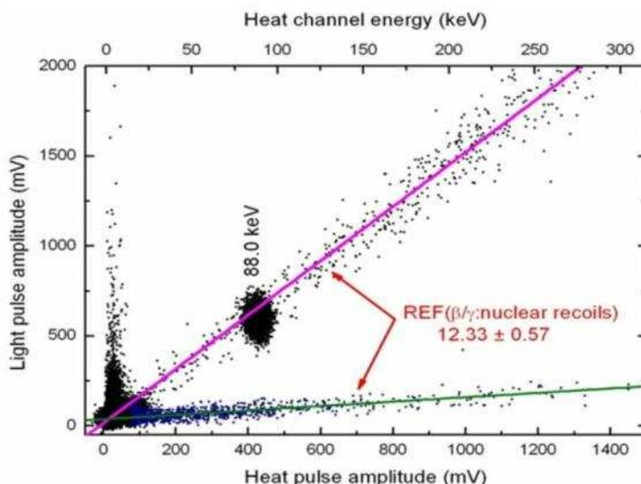
Fig. 4. Light versus heat discrimination plot in the 46 g BGO detector under a  $^{252}\text{Cf}$  neutron irradiation. The 88 keV line following EC at the  $^{207}\text{Pb}$  K-shell dominates and is well separated from the nuclear recoil events while the 15 keV lines (L-shell) could limit the detector discrimination threshold.
