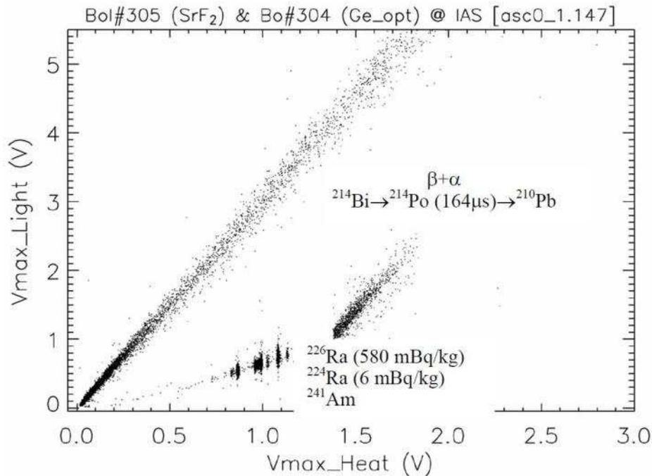
Fig. 7. Background in a 54 g SrF<sub>2</sub> bolometer at IAS which evidences the presence of a high contamination in the natural radioactive chains. A <sup>241</sup>Am source was added for calibration purposes.
