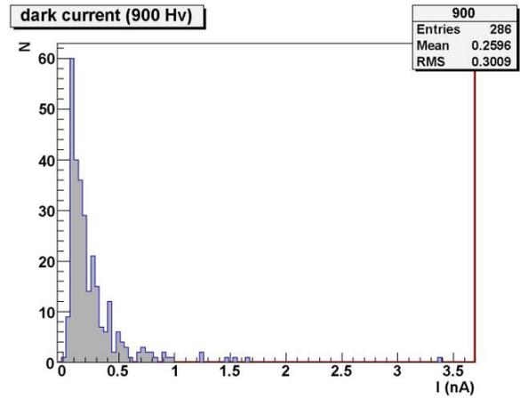
Fig.6. Dark currents of PMT’s in HV=900 volts.
