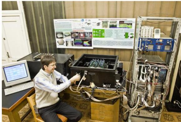
Fig.2. The general view of the PMT testbench: left – "Light Box", center – "PMT Box", right – "Electronics Rack".
