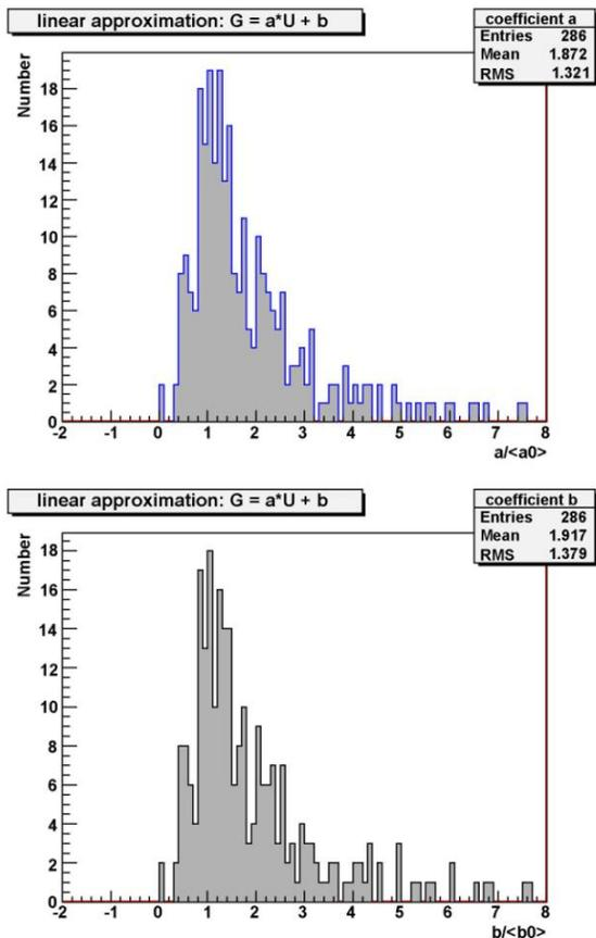
Fig. 5. The “a” and “b” coefficient distribution of linear approximation of the gain curve for each PMT.
