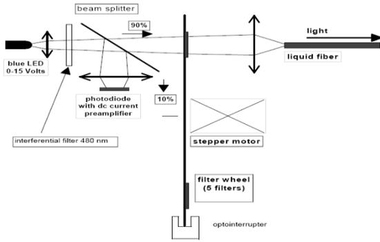
Fig.4. The PMT calibration optical scheme.
