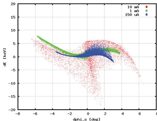
Figure 4: Longitudinal phase space of the 5 MeV beam exiting MAMBO at several beam currents.  $I_b = 150 \mu\text{A}$  (blue), 1 mA (green) and 10 mA (red).
