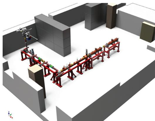
Figure 5: Test setup of STEAM, MELBA and MAMBO No. 1 & No. 2 in the MEX-3 hall. For a better overview the supports of STEAM are suppressed.
