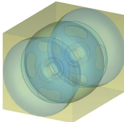
Figure 1: Geometry used for multipacting simulation.
