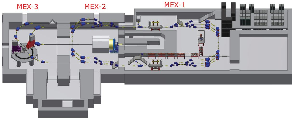
Figure 2: Layout of the MESA facility with the new MESA experimental hall 1 (MEX-1) on the right hand side and the two existing halls on the left-hand side, now renamed to MESA experimental hall 2 and 3 (MEX-2 and MEX-3).
