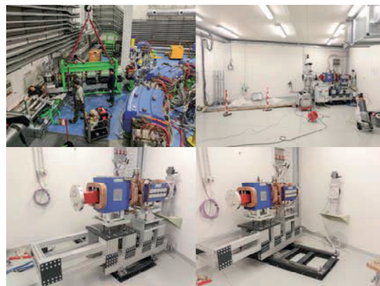
Figure 8: Status of installation of XPR optics line. Up left: XPR line in the synchrotron hall; up right: XPR room at actual state; down: scanning magnets positioned on the beam line (left) and moved out of the beam line (right).
