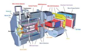
The Detector is composed of two magnetic spectrometers- Target Spectrometer (TS) and Forward Spectrometer (FS). There are three sub detectors (MVD, STT, GEM) for tracking, Electromagnetic Calorimeter (EMC), a muon system and Cherenkov Detectors (RICH, DIRC) and a time-of-flight (TOF) system [2] as shown in the figure1.
