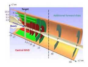
Fig.2 Micro Vertex Detector with lambda disks
