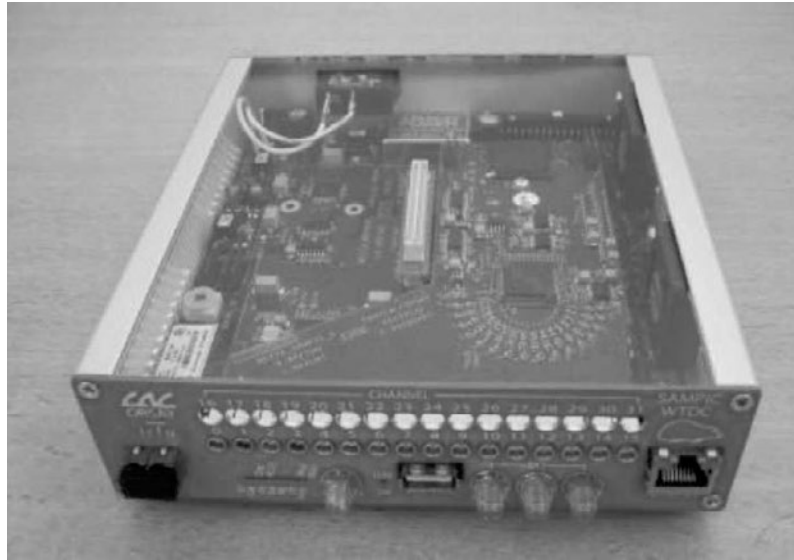
Figure 74: Picture of the SAMPIC chip and its acquisition board.
