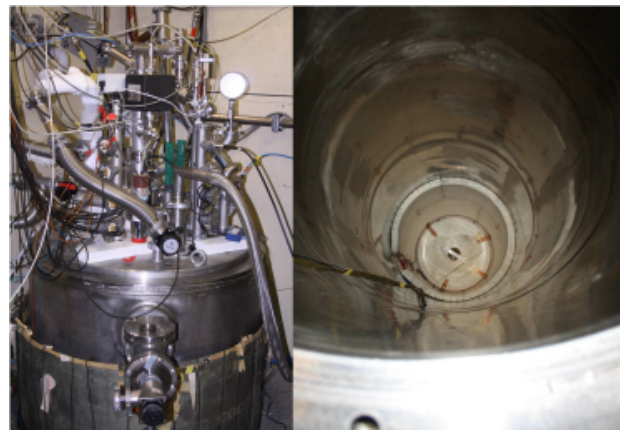
Figure 1: Left: upper part the vertical cryostat. Right: top view of the cryostat internal surface.
