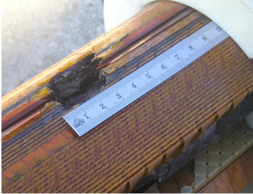
Figure 2.17: Damage of a dipole coil after a quench during tests. The 7 MJ stored in the magnet were released in one point of the coil due to an interturn short-circuit (production imperfection).
