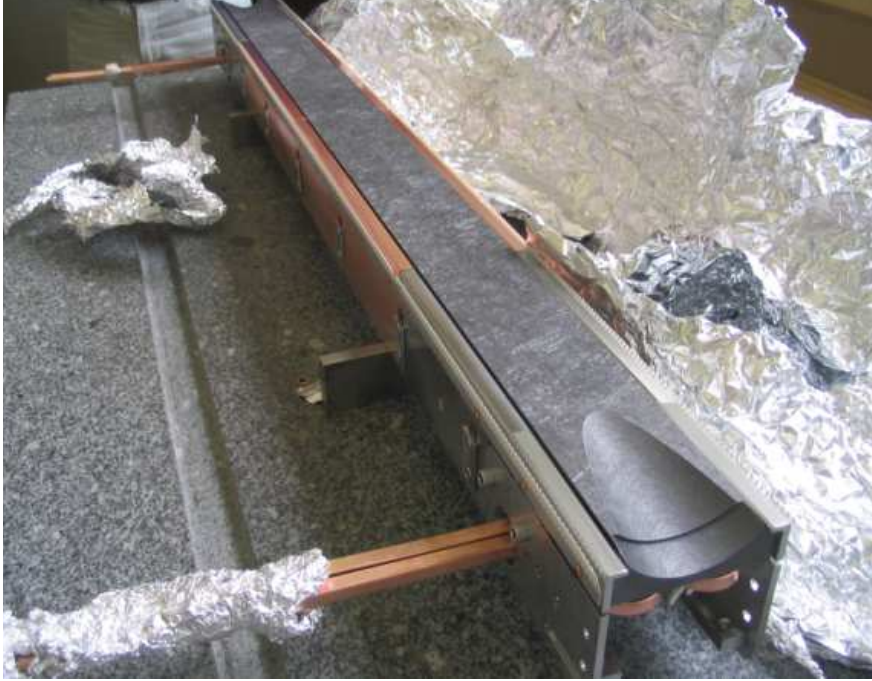
Figure 2.11: Carbon collimator jaw used in LHC collimators.
