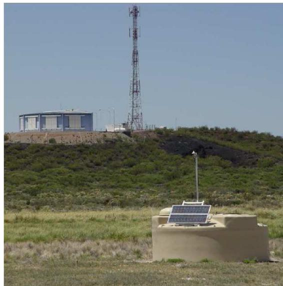
Figure 2.4: Surface detector station with solar panel GPS and communication antenna in the foreground. In the FD building the shutters for the telescopes are closed. The antenna next to the FD building is connected to the data acquisition system of the SD array.
