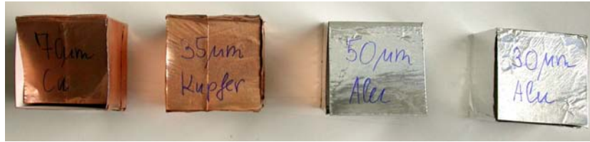
Figure 7.64: Selection of boxes used to shield a detached L_AirCore PCB.
