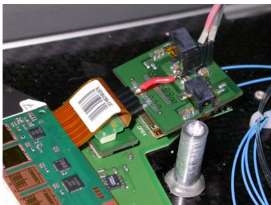
(a) Directly connected to the ICB via a bridge connector.
