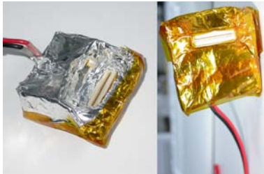
Figure 7.66: Top and bottom sides of a L_AirCore PCB shielded with aluminium. The bottom side is isolated with Kapton tape.
