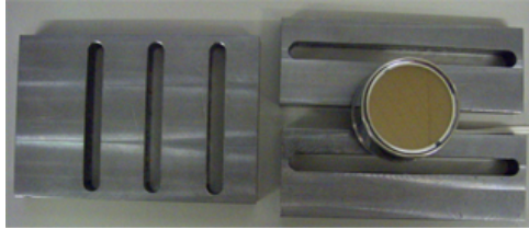
Figure 7.1: Lead collimator with 1.8 cm thickness in 2008 (a 2-inch PMT is shown for a reference). The lead on the left side has vertical slits of 1 cm width and the two leads on the right side have a 13 cm-length horizontal slit. Between two leads with the horizontal slit, another collimation is possible by these gap as shown in picture. The lead with horizontal slits in 2009 has a three times longer length.
