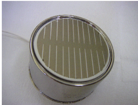
Figure 3.35: Photo-multiplier tube for the LXe detector. Aluminum stripe makes a flat response.
