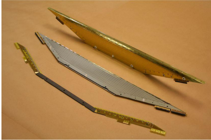
Figure 3.19: Element of a drift chamber module.
