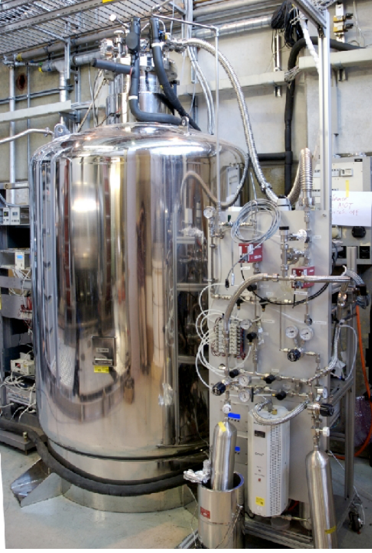
Figure 3.47: Liquid xenon tank and gaseous purification system.
