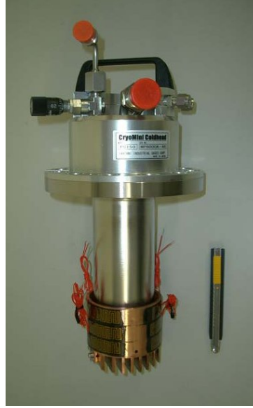
Figure 3.45: Pulse tube refrigerator for liquid xenon.
