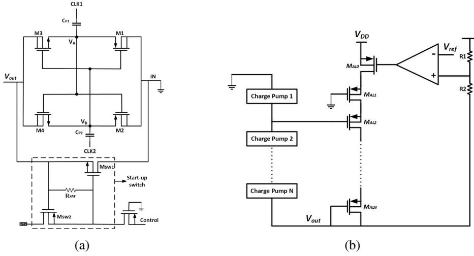
**Figure 4.** (a) Schematic of 1-stage charge pump. (b) Block diagram of closed-loop charge pump.  $V_{ref}$  is the reference voltage which is set to 1 V.
