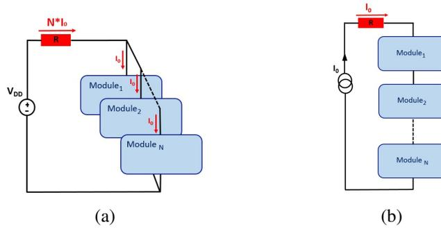
**Figure 1.** (a) Block diagram of parallel powering scheme. (b) Block diagram of serial powering scheme.
