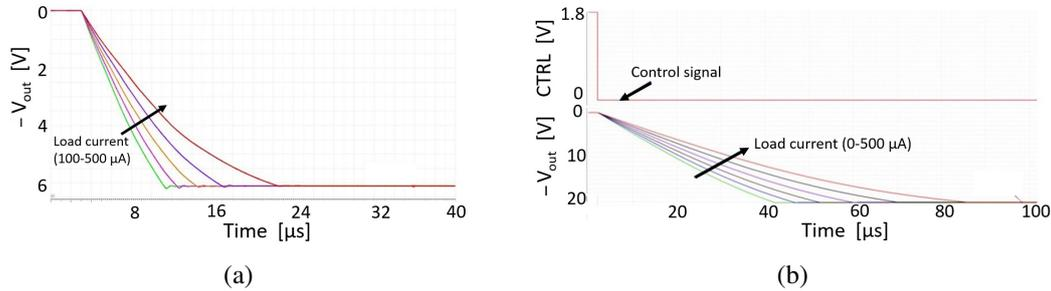
**Figure 6.** (a) (b) Closed-loop output voltages of 6-stages and 19-stages charge pump for various load currents with the pumping frequency of 640 MHz.
