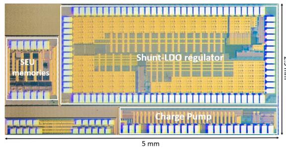
**Figure 2.** Die photograph of the three blocks: Shunt-LDO regulator, charge pump and single event upset (SEU) tolerant memories. All three test circuits are for the same detector in TJ CMOS technology.
