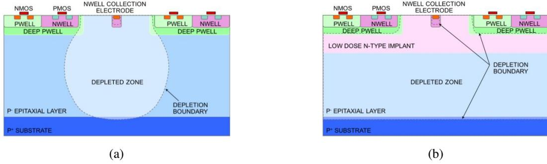
**Figure 3.** (a) The standard TJ 180 nm CMOS process. (b) The modified TJ 180 nm CMOS process. Reproduced from [9]. CC BY 4.0.
