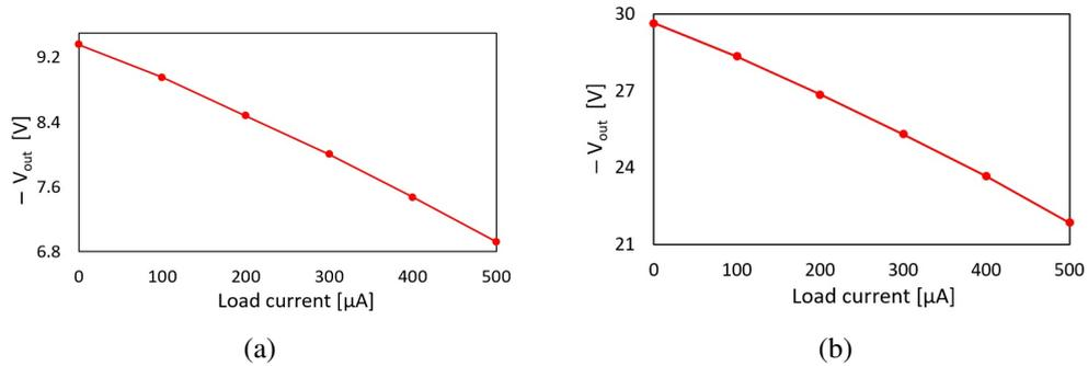
**Figure 5.** (a) (b) Output voltage characteristics of the open-loop 6-stages and 19-stages charge pump as a function of the load current with the pumping frequency of 640 MHz.
