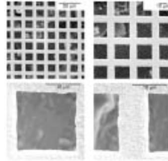
Fig. 3. Detailed pictures of Buckbee-Mears electro-mesh used to construct the Micromegas detector. The mesh has 1000 lpi., has square holes of  $17 \times 17\mu\text{m}^2$ , and a  $9\mu\text{m}$  wide wall separating them.
