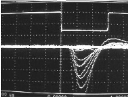
Fig. 6. Typical single electron pulses from this detector together with a QVT gate. A charge integrating amplifier has a gain of  $2.7 \text{ V/electron}$ , and a shaping time of 65ns.
