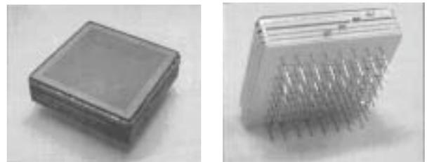
Fig. 13. A possible future step is to build the proposed detector in the already well proven structure, for example, in the Burle MCP-PMT enclosure.
