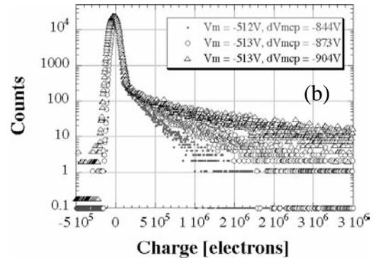
Fig. 7. Single electron pulse height spectra in 89.1% He + 10.9%  $i\text{C}_4\text{H}_{10}$  gas: (a) vary the “bottom” power supply, which controls both the Micromegas and MCP gain, and (b) vary voltage  $dV_{mcp}$  across the MCP.
