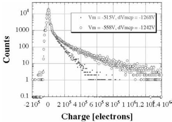
Fig. 10. Single electron pulse height spectra in 96% Ar + 4% CH<sub>4</sub> gas
