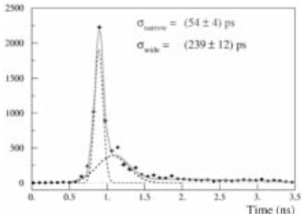
Fig. 1. Single electron timing resolution obtained with a vacuum-based Burle MCP-PMT, and PiLas red laser diode. The MCP-PMT has Two micro-channel plates (MCP or Capillary). This measurements indicates that there is a good transit time distribution in the vacuum-based capillary. A long tail is explained by the recoil photoelectrons from the front MCP surface.
