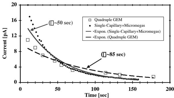
Fig. 12. The charging effects in the structure was measured using a strong Mercury lamp creating a standing current of  $350\text{nA}$ , which was suddenly interrupted to measure the discharging time constant. We measure a time constant of  $\sim 50\text{sec}$  for the presented detector, and this is to be compared to  $\sim 85\text{sec}$ , which was measured for the Quadruple-GEM detector [9].
