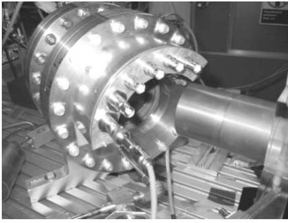
Fig. 5. Experimental setup with Hamamatsu UV Xe lamp L2435. The UV light is focused on a small spot on the dense s.s. mesh to produce the single electron source.
