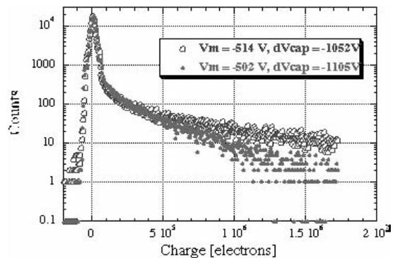
Fig. 9. Single electron pulse height spectra in 94.5% He + 4.5%  $\text{CH}_4$  gas.
