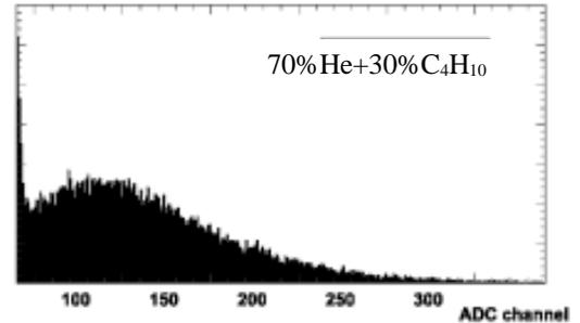
Fig. 8. Single electron pulse height spectrum measured in a Micromegas in 70% He+30%  $i\text{C}_4\text{H}_{10}$  [8].
