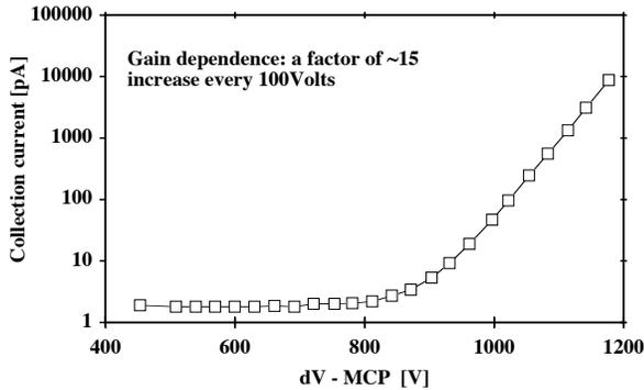
Fig. 11. Absolute gain measurement in MCP in 94.5% He + 4.5% CH<sub>4</sub> gas. The MCP was in collection mode and the light source was a strong Mercury lamp. A gain increase by a factor of  $\sim 15$  every 100 Volts was observed. A similar gain was measured in the Micromegas in the same gas.
