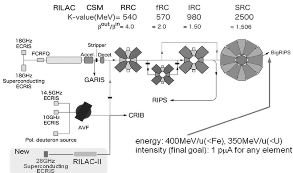
The condition of a stripper foil, which is placed immediately after RRC, is the severest, and a thin rotating carbon foil is used. Damage by the uranium beam is enormous: it may make a big hole after a several-hour operation. The carbon foil stripper was replaced by a helium gas stripping system at the beginning of 2012. The charge state was lowered by this replacement, and a minor alteration was done at fRC.
