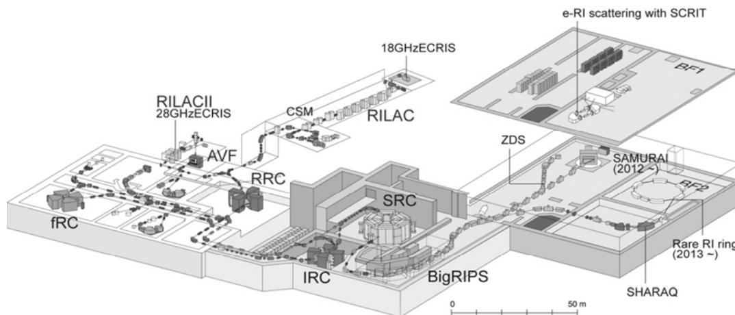
The accelerated beam is conducted into BigRIPS (big RIKEN projectile fragment separator) [4], where any nuclide lighter than uranium can be produced. The secondary unstable beam is delivered to the experimental area.
