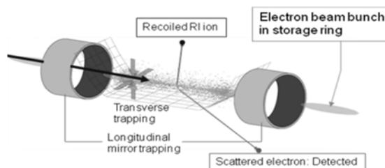
**Figure 4: Layout of the SCRIT facility**
