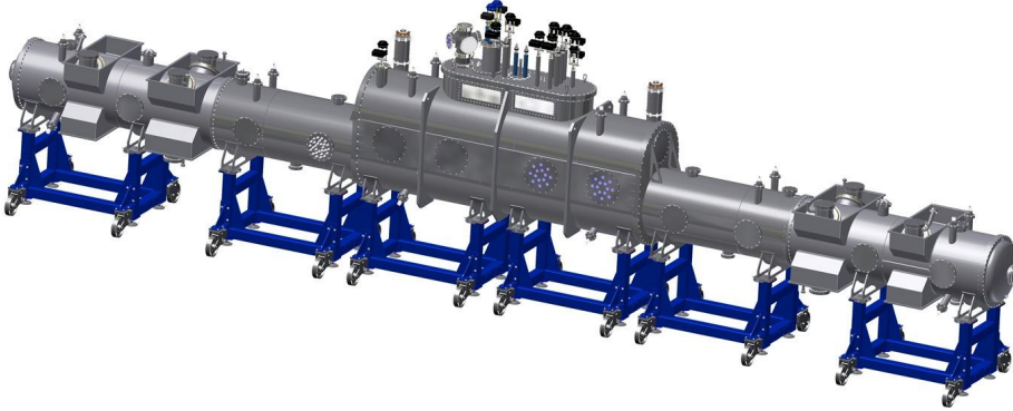
Figure 2.4: CAD drawing of the WGTS including the DPS-1F and DPS-1R on separate stands.
