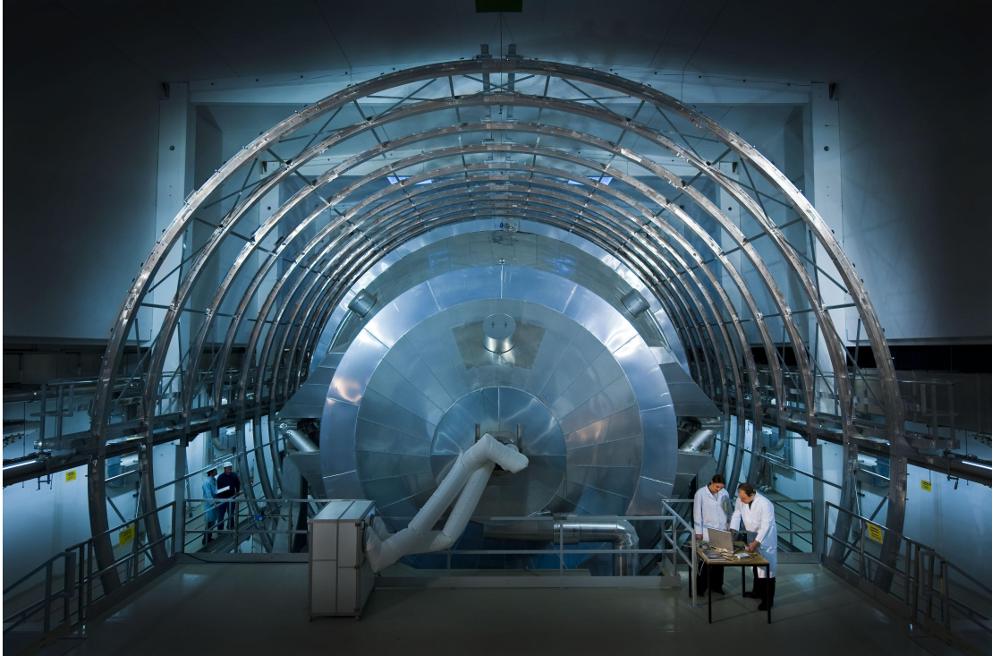
Figure 2.9: The KATRIN main spectrometer surrounded by the air coil system. (photo: KIT)
