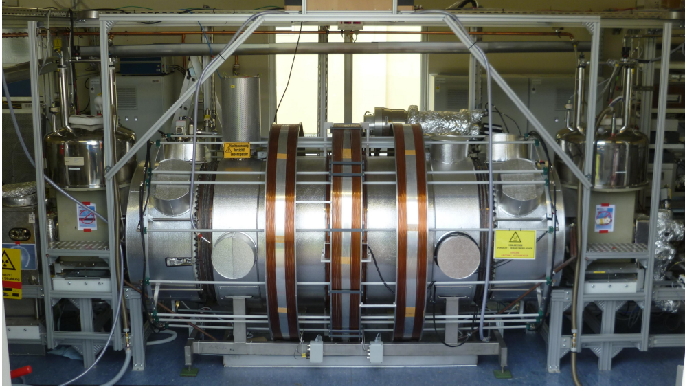
Figure 2.10: Picture of the operational monitor spectrometer which is the repurposed setup of the Mainz experiment. It has two solenoids and three aircoils. (photo: M. Erhard [140])
