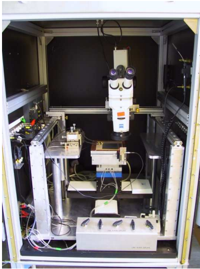
(a) QTC-probe station for the electrical tests on the sensors
