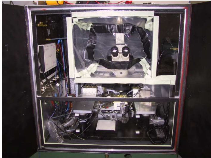
(b) IQC-probe station with humidity shield for operation at -10^{\circ}\text{C}
