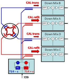
Figure 6: BPM calibration system.
