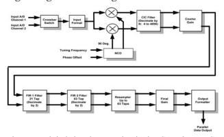
Figure 7: Digital signal processing in the *Graychip* DDC. Key to the digital signal processing is the 4 channel GC-4016 ASIC (*Graychip*, see Figure 7), which is part of the 8-channel *Echotek* digital receiver VME board. Each signal is digitized at 69.24 MS/s, generating 32 samples / turn. This DDC input data is I-Q demodulated (NCO), low-pass filtered, and decimated using CIC and FIR filters
