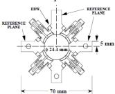
Figure 3: ATF damping ring button BPM.
