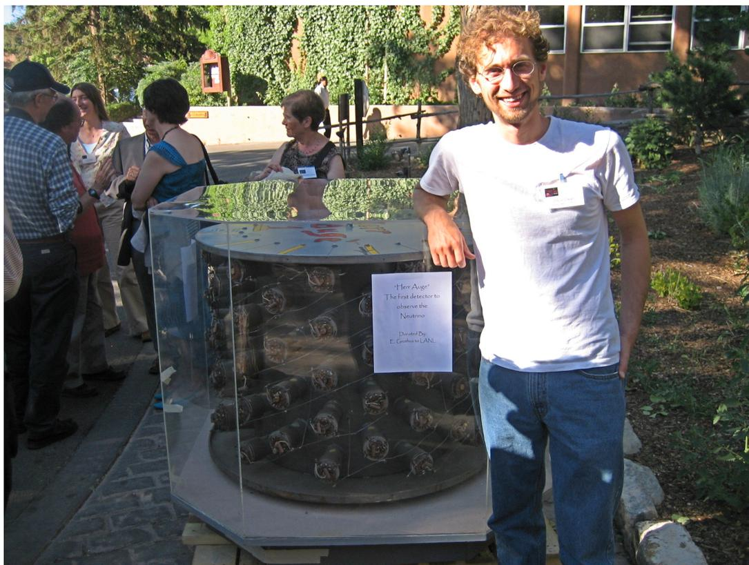
Figure 3.5: The Hanford antineutrino detector, also known as Herr Auge (Mr. Eye). The detector consisted of a 300 l cylindrical tank of liquid scintillator instrumented with 90 photomultiplier tubes. The bases of the photomultiplier tubes can be seen behind the acrylic display case.
