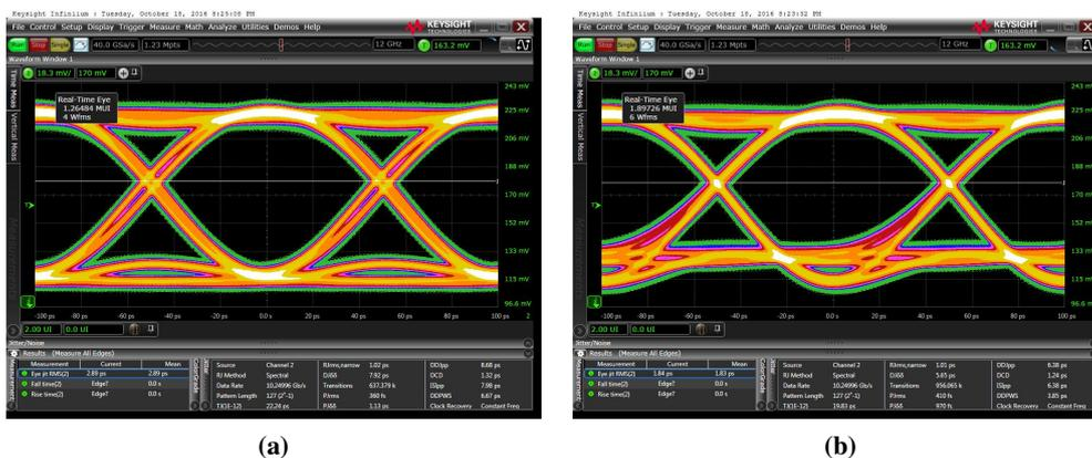
**Figure 10.** 10 Gb/s optical eyediagrams with (a) no pre-emphasis (b) pre-emphasis on.
