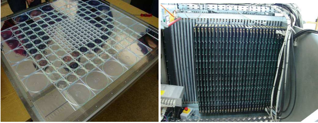
Figure 1: Picture of one AHCAL active layer (left) and of AHCAL the steel stack support with active layers installed (right).
