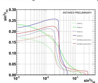
Figure 3: Expected upper limits at 90% (dashed red) and 99% (solid red) C.L. for the analysis of our pseudodata sample. Exclusion regions are on the right side of the lines. For comparison limits from IceCube [19], and from Super Kamiokande [20] are also shown.
