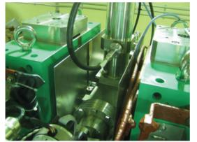
Figure 4: View of magnetic shield installed between the body and coil and on the body surface.
