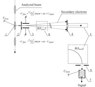
Figure 1: Principal of BSM (1: target, 2: input collimator, 3: RF deflector combined with electrostatic lens, 4: output collimator, 5: bending magnet, 6: collimator, 7: Secondary Electron Multiplier, 8: steering magnet)
