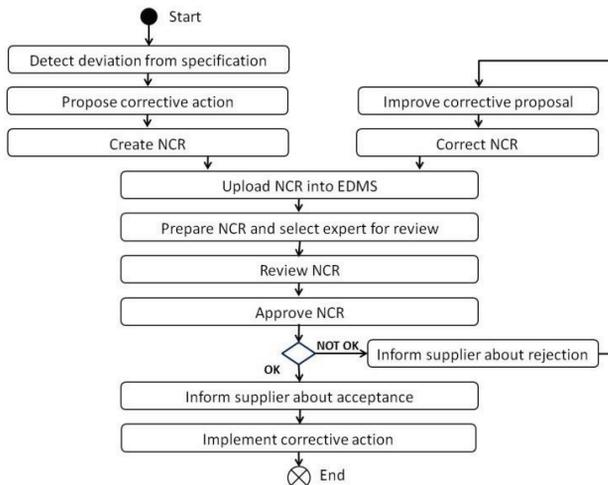
Figure 3: Cavity non-conformity life-cycle.
