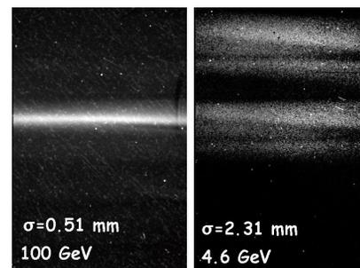
Figure 3: Fluorescence image profile and the width of RHIC Au ion beams.
