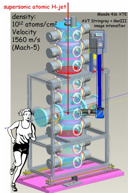
Figure 1: H-jet with external modification including the attachment of an optical imaging system (not to scale).
