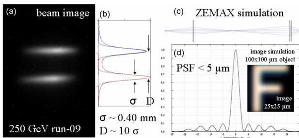
Figure 4: (a) 250 GeV proton beam image and (b) the corresponding width of the blue and yellow beams. (c) ZEMAX optical simulation of the imaging system and (d) the PSF, inset shows the image simulation.
