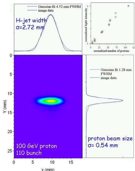
Figure 2: False color fluorescence image profile for a RHIC proton beam, 656 nm filtered. The x and y projections of the image profile correspond to the width of the H-jet and the vertical beam size, respectively. The brightness of the fluorescence increases linearly with proton beam intensity.
