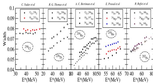
FIG. 1: Width as a function of compound nucleus excitation energy for various systems [1–5].
