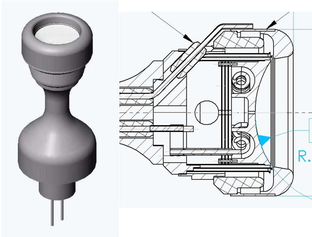
**FIGURE 6.** Model of gun stem and layout drawing of cathode stem assembly.
