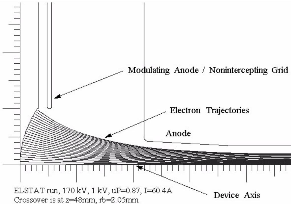
**FIGURE 1.** On-axis simulation of electron gun at 170 kV, 60 A.
