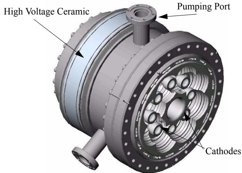
**FIGURE 7.** Solid model of complete electron gun for beam analyzer testing.
