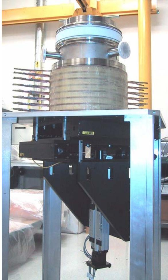
**FIGURE 12.** Precision support hardware for beam analyzer current probe
