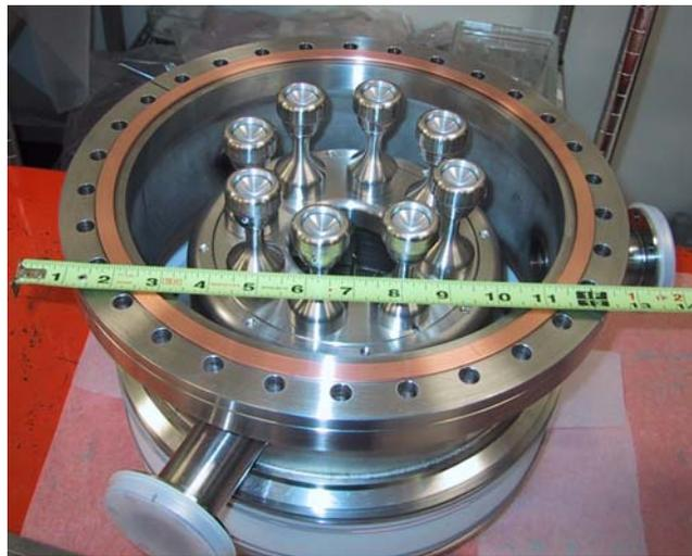
**FIGURE 8.** Photograph of the cathode stem assembly mounted in the gun vacuum envelope.
