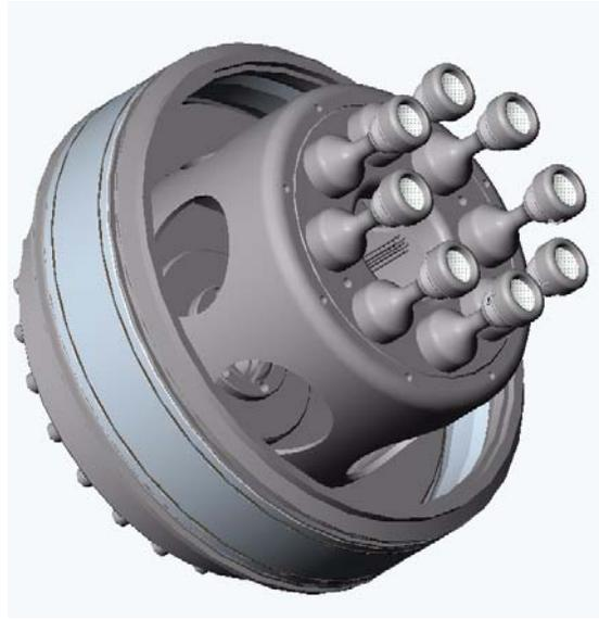
**FIGURE 2.** Configuration of electron guns for eight beam multiple beam gun.
