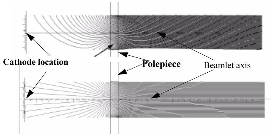
**FIGURE 3.** Uncorrected and corrected magnetic flux lines for off-axis electron guns.
