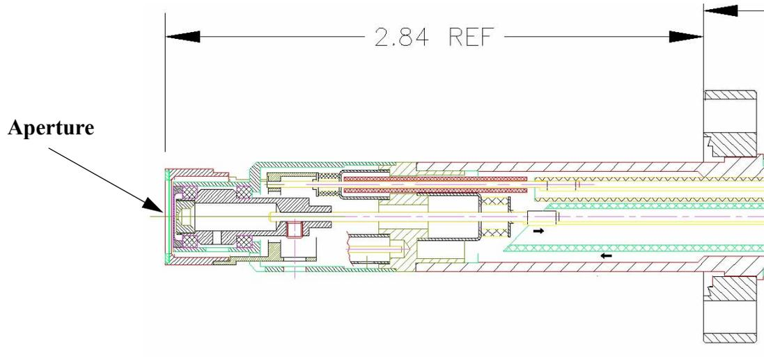
**FIGURE 11.** Cross section view of beam analyzer current probe.
