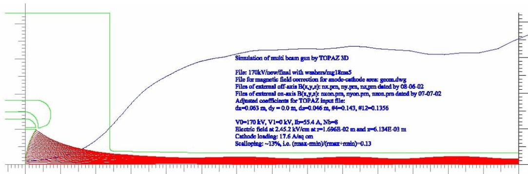
FIGURE 5. 3D beam simulation results for one beamlet of eight beam multiple beam gun.
