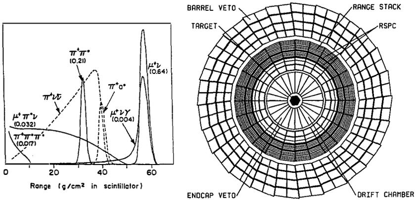
**Figure 2.** a) Charged-track range spectra for  $K^+$  decays. b) The E-787 spectrometer, end view. The beam enters along the axis (at right angle to the page).
