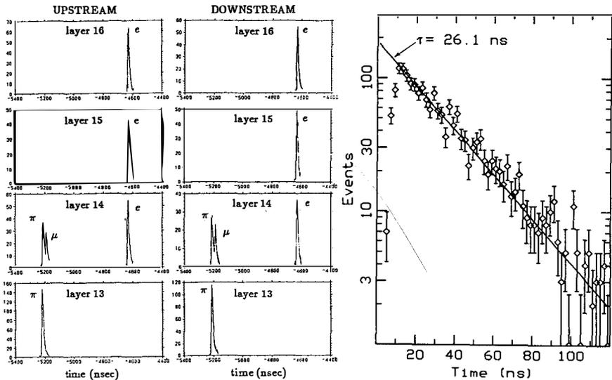
**Figure 3.** a) Transient digitizer signals for a  $\pi^+$  stopping in the range stack. b) The  $\pi^+$  lifetime spectrum from TD pulse fitting.
