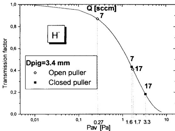
Figure 6. Transmission factor versus average pressure for slit<sub>PIG</sub> diameter of 3.4 mm.
