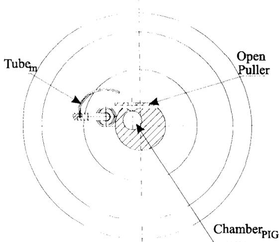
Figure 2. Experimental model of a cyclotron central region with "open" puller.
