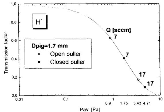
Figure 5. Transmission factor versus average pressure for slit<sub>pig</sub> diameter of 1.7 mm.
