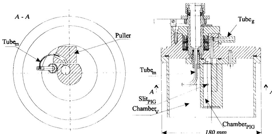
Figure 1. Experimental model of a cyclotron central region with "closed" puller.
