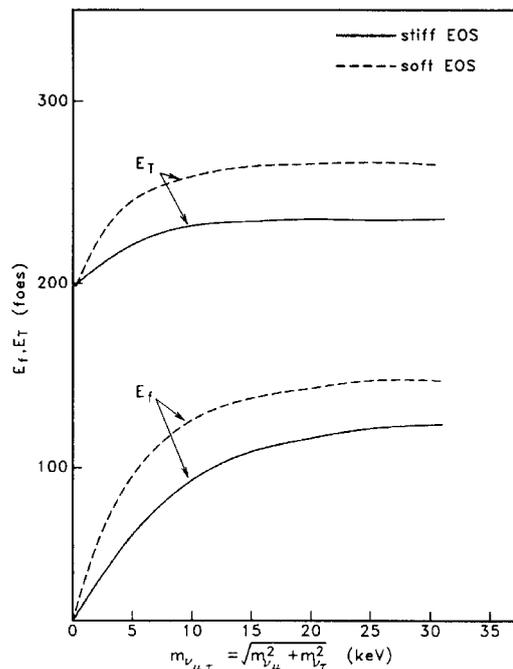
Fig. 2: The total energy released in all types of neutrinos,  $E_T$  and the energy lost via flipped neutrinos,  $E_f$ , as a function of  $m_{\nu_{\mu,\tau}}$  for both stiff and soft equations-of-state.
