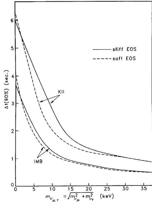
Fig. 4: The time taken for the accumulated number of events to reach 90% of the final total number of events as a function of  $m_{\nu_{\mu,\tau}}$ , for both detectors and both models.
