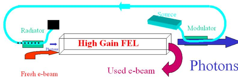
Figure 4 System diagram of the “Optics Free” FEL Oscillator.
