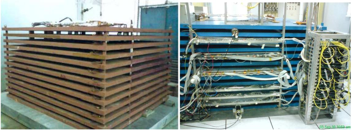
Figure 3.1: Left Panel: The INO iron calorimeter prototype detector at VECC. Right Panel: Six RPCs placed inside the iron layers, four of them are glass RPCs and other two are bakelite RPCs.
