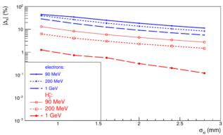
Figure 1: Space charge effects (given as deviation between the beam width input in the simulations and the one obtained by running the code) for different  $\sigma_{xi}$  (i.e. input  $\sigma_x$ ) and incident beam energies when  $\sigma_v = \sigma_z = 2$ mm and  $\mathbf{E} = \mathbf{E}_v$ = 300 kV/m.
