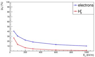
Figure 2: Comparison between the space charge effects for electrons and singly ionised hydrogen molecules  $H_2^+$ , for a 90 MeV proton beam with beam size  $\sigma_x = \sigma_y = \sigma_z = 2$  mm in an homogeneous electric field.
