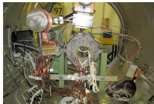
Fig. 11. Magnet package combined with current leads and thermal sinks.
