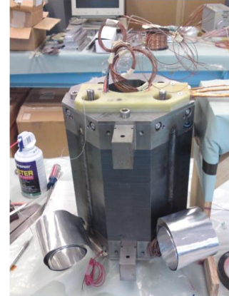
Fig. 4. The quadrupole magnet package cold mass.
