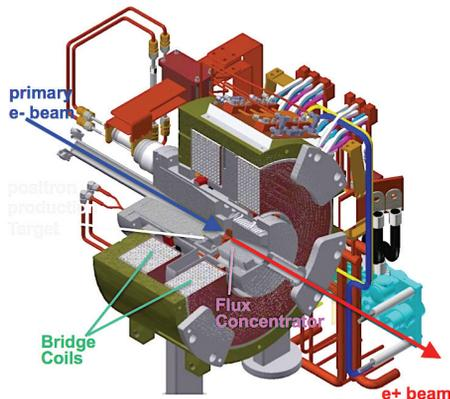
Figure 4: Flux concentrator assembly.
