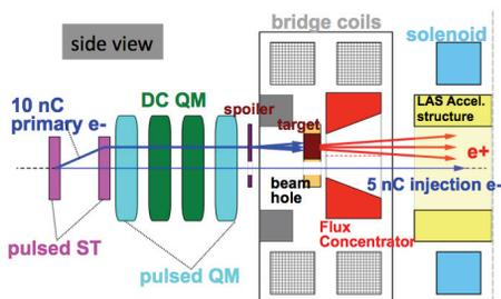
Figure 5: Positron target and a hole in front of FC and LAS.
