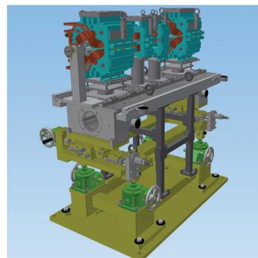
Figure 7: Girder design with precise alignment movers.
