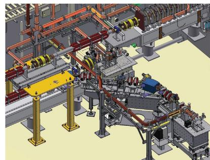
Figure 2: Birdview of straight and 90-degree photo-cathode RF-guns and a thermionic gun at the top.
