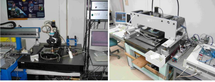
Fig. 5. The European (left) and Japanese (right) scanning systems.
