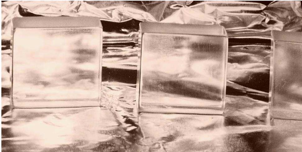
Figure A.2: New CsI(Tl) crystals in the process of being polished. The crystals are  $4 \times 4 \times 1$  cm<sup>3</sup> blocks of scintillating material providing high photon yield for PIN-diode readout.
