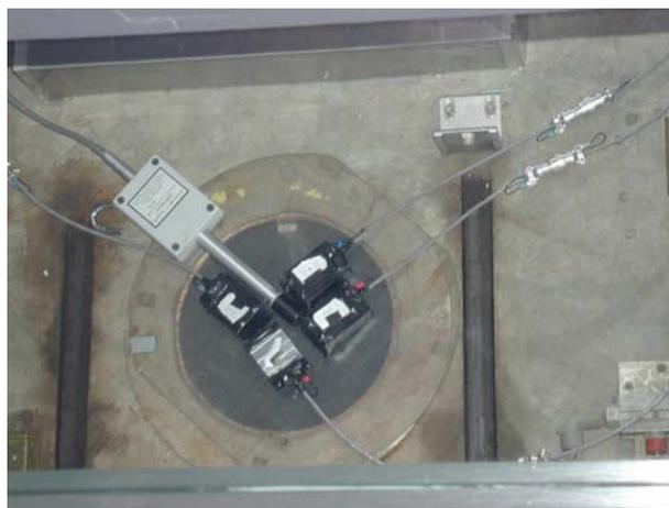
Figure A.7: Calibration in Co60 Source well, “aerial view”. Four sensors are seen on a sheet of Plexiglas on the top of the well. The radiation level is measured with a radiation meter (Radcal).
