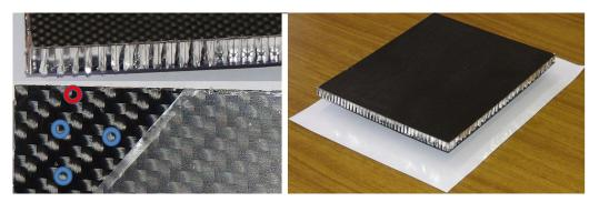
**Figure 5:** Samples of carbon plastic mirror. Left: flat sample, on top - three layer construction, on bottom - edge of the sample with 4 "points" for roughness estimations (reflective surface partially covered by protective film). Right: sperical sample with sizes  $18 \times 20$  cm<sup>2</sup> and radius of curvature 741 cm.
