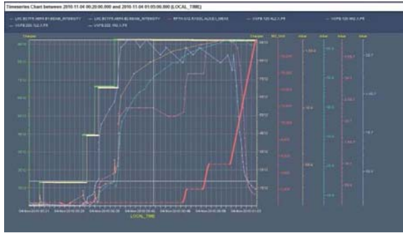
Fig. 9: Dynamic vacuum pressure rise close to the point 2 experimental area vs. injected beam current and ALICE solenoid current.
