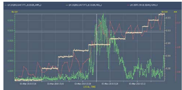
Fig. 1 : Beam size evolution (red) vs. time when the vertical tune frequency (ochre) is varied. The amplitude of the vertical oscillation (green) reached its maximum when the tune overlaps the hump tune (0.304). Courtesy R. Steinhagen.
