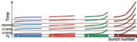
Figure 7: Example for a Mountain range type beam emittance display for the LHC beams. Time progresses along the vertical axis, starting with injection, and the horizontal axis identifies the bunch numbers.
