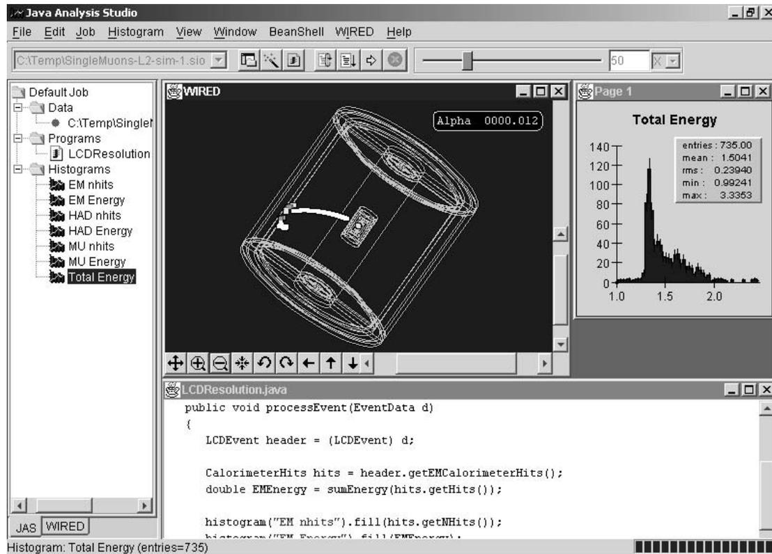
Figure 1 The JAS application showing histogram browsing, plot display, code editor and WIRED event display.
