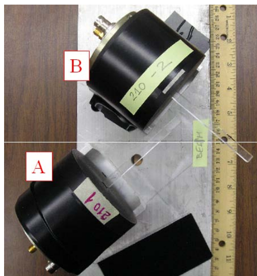
Fig. 17. Photek 210 with quartz radiators (bar's size 6x6x100 mm 3 ) aligned at 48° to the beam. The measured time difference is (t_A - t_C) + (t_B - t_C)/2 . The time jitter, due to the beam size in the horizontal direction cancels.
