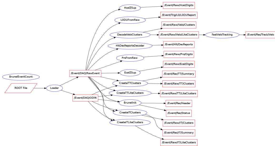
Figure 1. The algorithm state machine using in the forward scheduling implementation.
