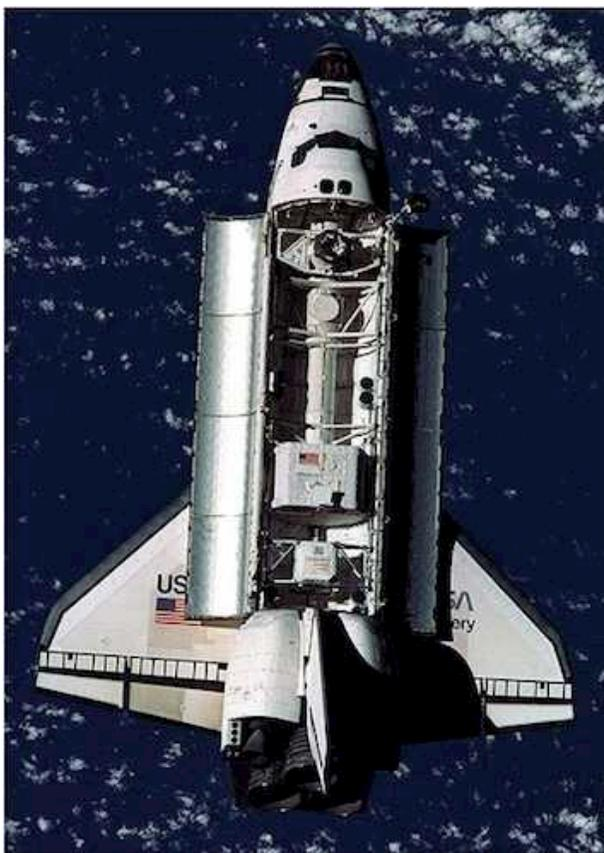
Figure 1.7.: The picture shows the cargo bay of the Discovery space shuttle in which AMS-01 detector was placed at the tail part of the cargo bay [64].
