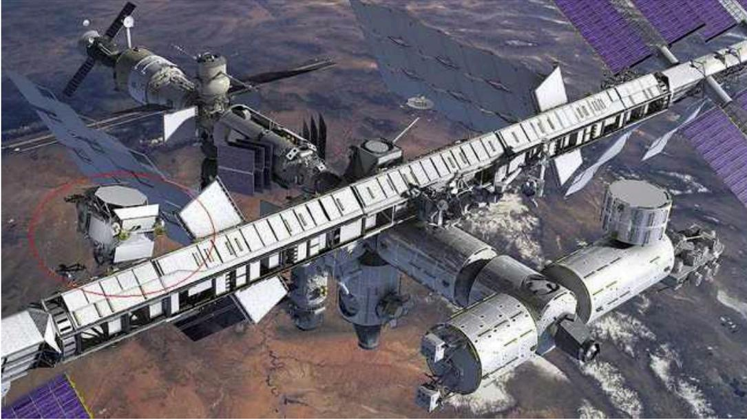
Figure 1.8.: The picture shows the AMS-02 detector (shown in the red circle). The detector has been installed at the International Space Station (ISS) [66].
