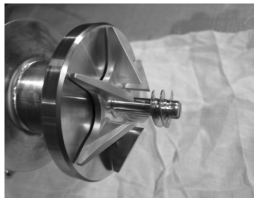
Figure 8 Liquid helium pump fitted with inducer
