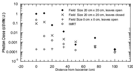
Fig. 5: Photon Dose (Aluminium Oxide) at different locations along the patient plane
