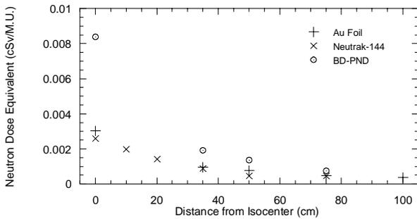
Fig 4: Comparison of neutron dose equivalents measured by different dosimeters
