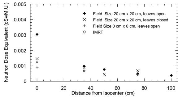
Fig. 1: Neutron dose equivalent (gold foil) at different locations along the patient plane.
