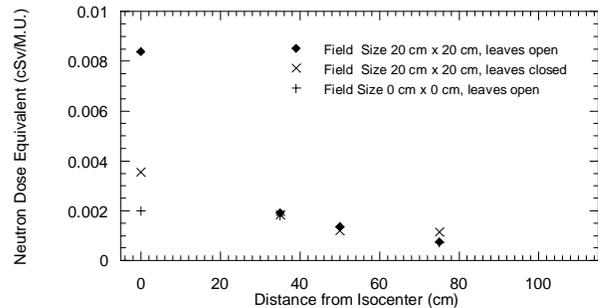
Fig. 3: Neutron dose equivalent (BD-PND) at different locations along the patient plane
