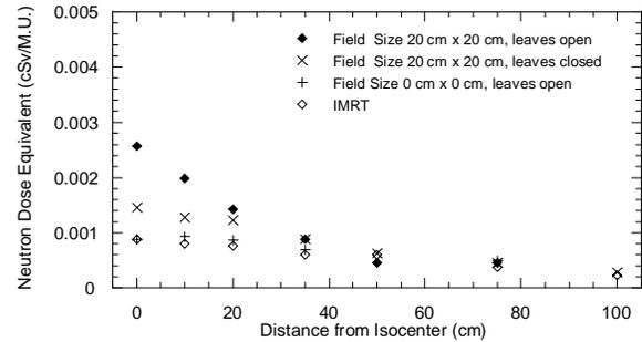
Fig. 2: Neutron dose equivalent (Neutrak-144) at different locations along the patient plane
