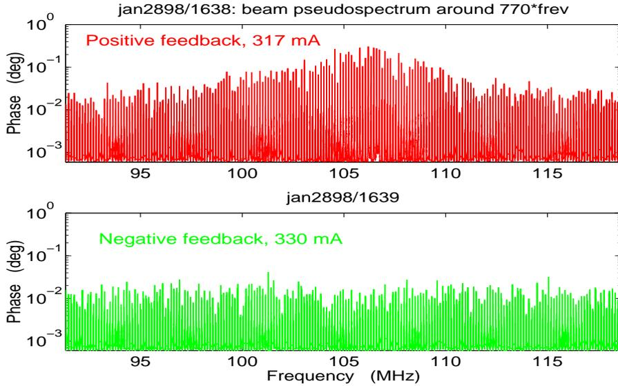
**FIGURE 1.** Beam pseudospectra with positive and negative feedback. Sidebands are driven up by positive feedback in the 100-110 MHz frequency range, which coincides with the aliased impedance of the 0-M-2 cavity HOM.
