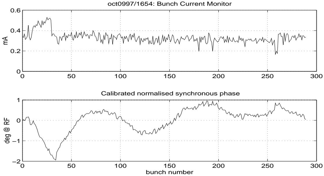
**FIGURE 3.** The upper figure shows the current variation in a 96 mA 291-bunch HER beam. We see a short impulsive discontinuity in the fill shape. This discontinuity produces a damped oscillation in the synchronous phase transient (lower figure). The transient completes 3 oscillations within the length of the bunch sequence.
