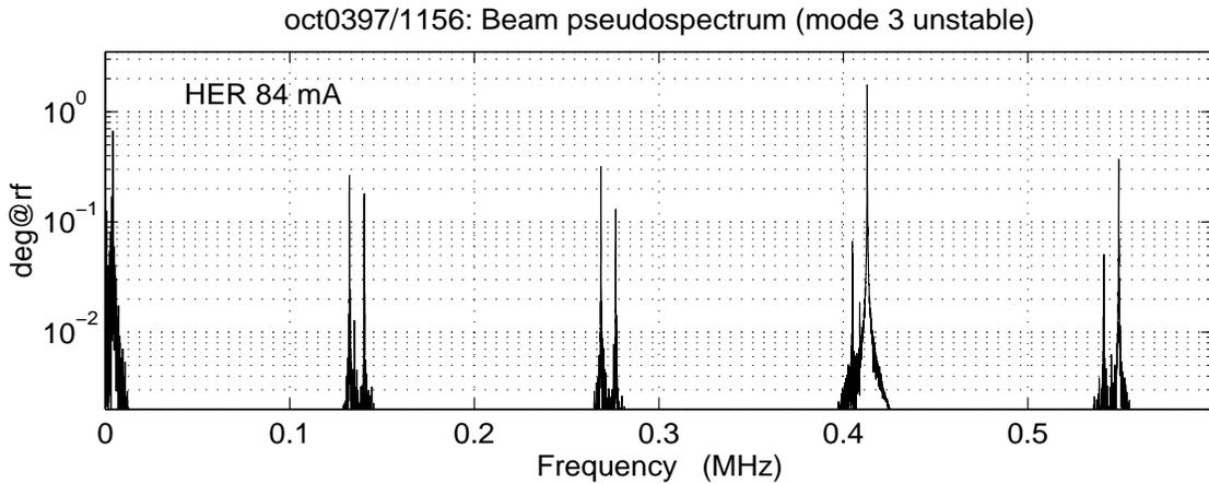
**FIGURE 5.** Beam pseudospectrum of 84 mA 291-bunch beam, showing an unstable upper sideband at the third revolution harmonic (0.41 MHz).
