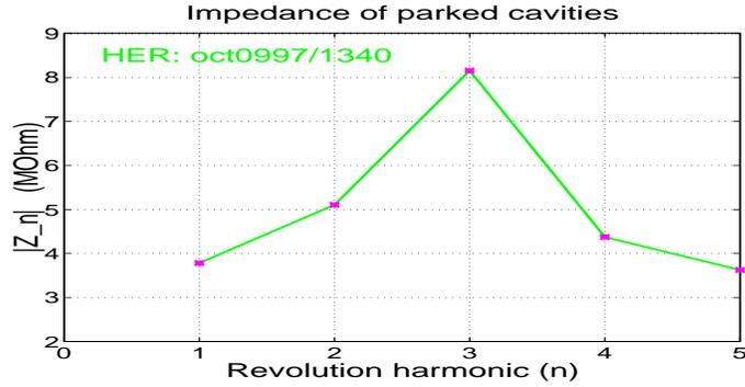
**FIGURE 4.** Impedance at first few revolution harmonics, extracted from bunch currents and synchronous phases. Large value at  $n = 3$  is due to the fundamental resonances of parked cavities.
