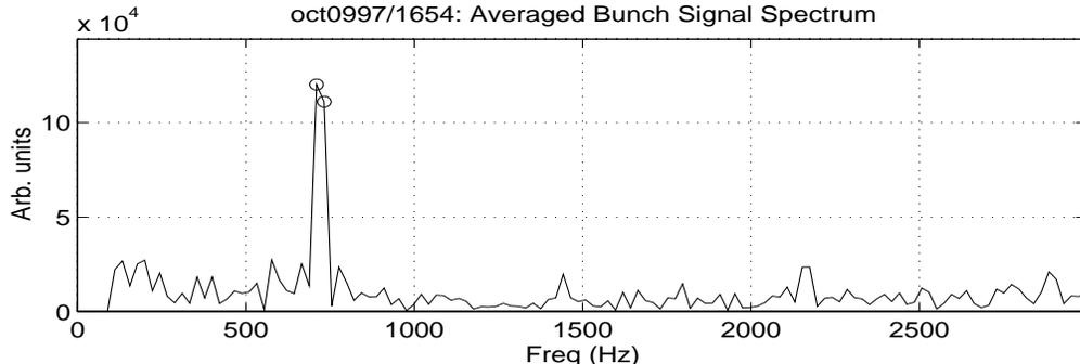
**FIGURE 2.** Low frequency bunch signal spectrum: 720 Hz line from klystron is demodulated to extract bunch currents from LFB system data.
