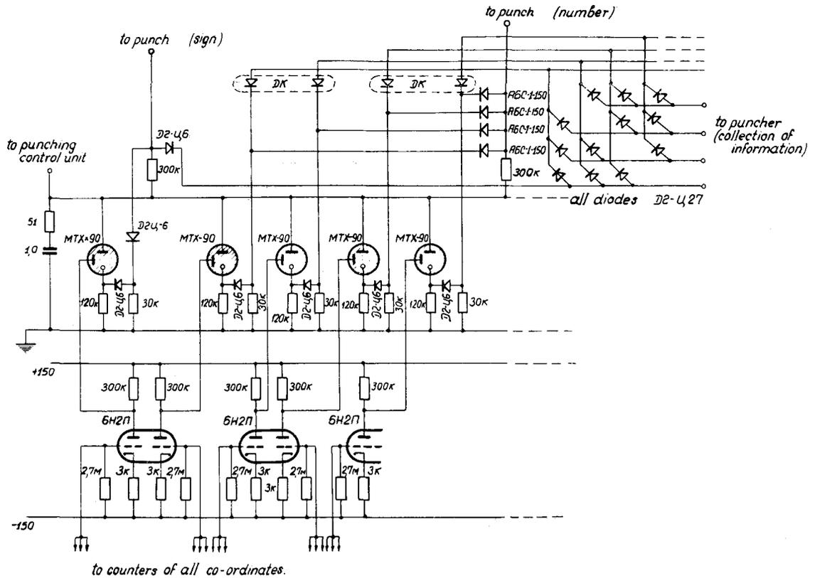
Fig. 8 The circuit diagram of the memory for a number and its sign.
