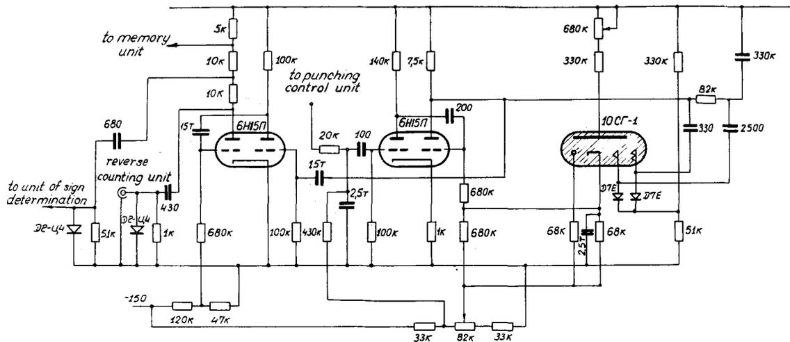
Fig. 9 The circuit diagram of the recording generator.
