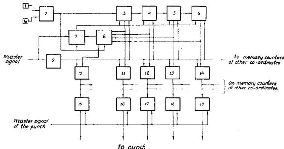
**Fig. 3** Block diagram of counting and recording device of the stereocomparator (for one co-ordinate).
