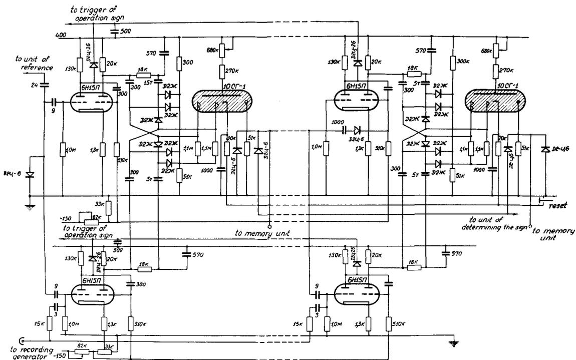
**Fig. 4** The circuit diagram of 1 and 4 type reversible dekatron counter.
