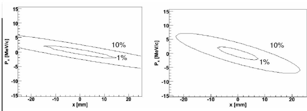
*Figure 7: Alignment tolerances at a position somewhere upstream of the spectrometer solenoid. On the left, tolerances are shown for the condition that  $r$  is within tolerance at the tracker reference plane. On the right, tolerances are shown for the condition that  $p_t$  is within tolerance at the tracker reference plane.*
