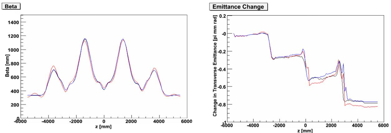
Figure 4: beta function and transverse emittance evolution for a muon beam in the presence of angular momentum (black) 0 canonical angular momentum (red) 10% reduction in kinetic angular momentum (blue) 10% reduction in kinetic angular momentum, rematched.
