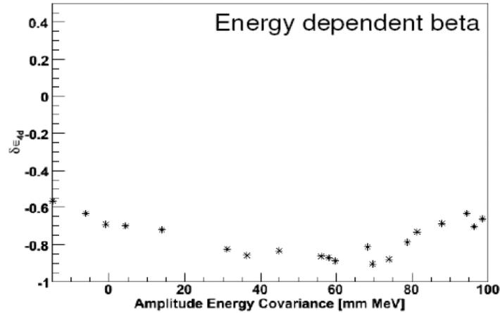
Figure 6: Effect of applying beam matching at different momenta on the transverse cooling performance together with an amplitude energy correlation.
