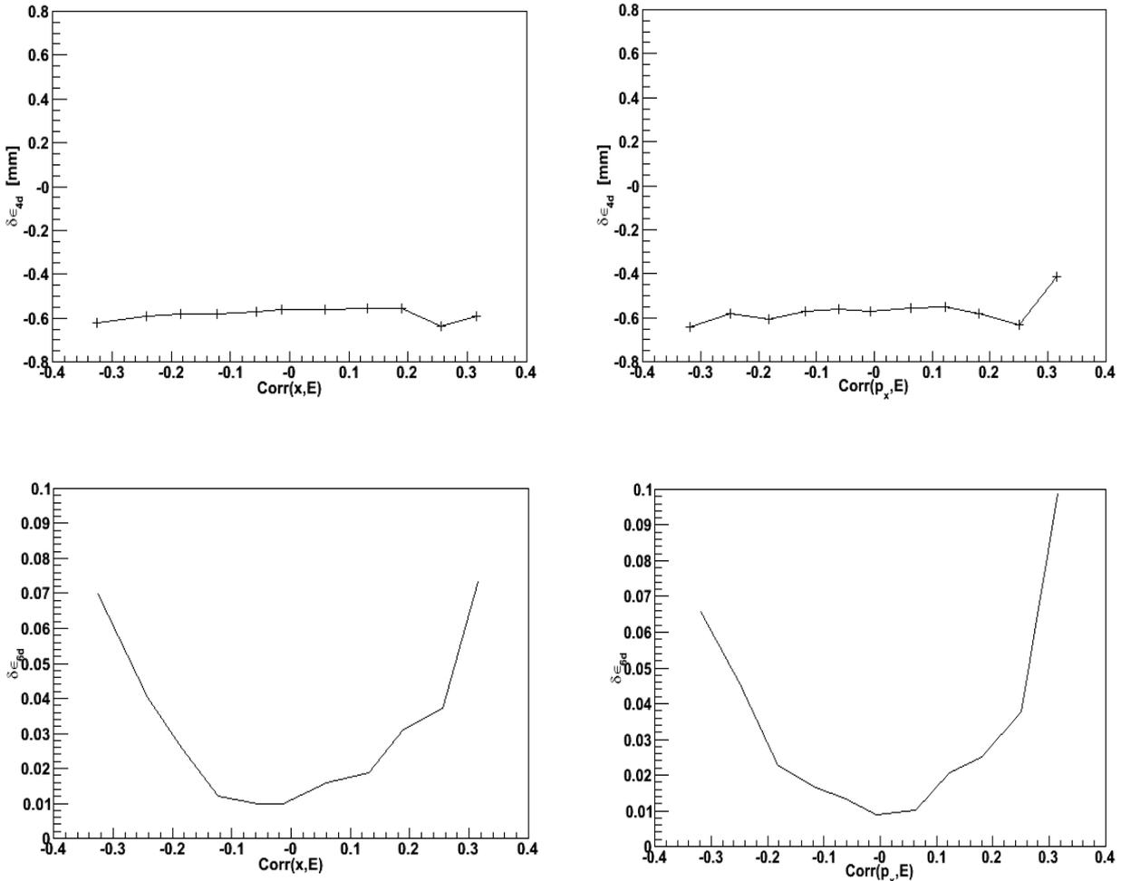
Figure 3: Effect of longitudinal-transverse correlations on cooling performance. (Top) 4D cooling performance (Bottom) 6D cooling performance (Left) correlation between  $x$  and  $E$  (Right) correlation between  $p_x$  and  $E$
