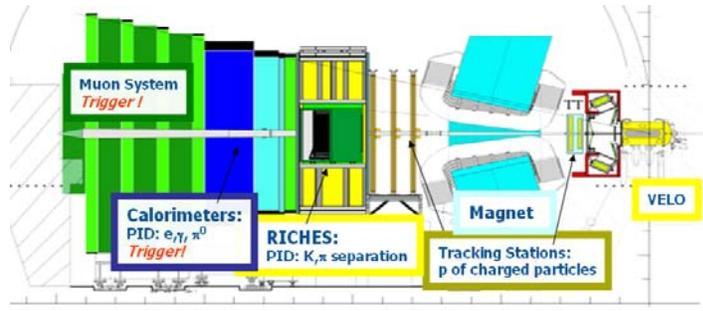
Fig. 4. The LHCb experiment's detector.
