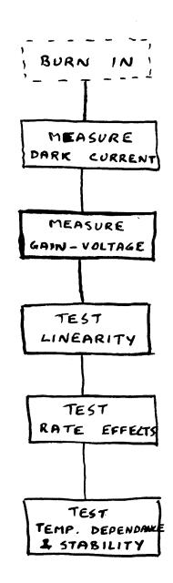
PMT TEST PLAN
