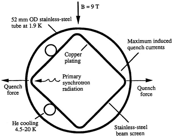
FIGURE 4: A schematic diagram of the square-section beam screen.
