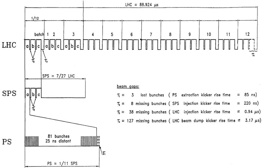
FIGURE 3: Bunch disposition in LHC, SPS and PS.
